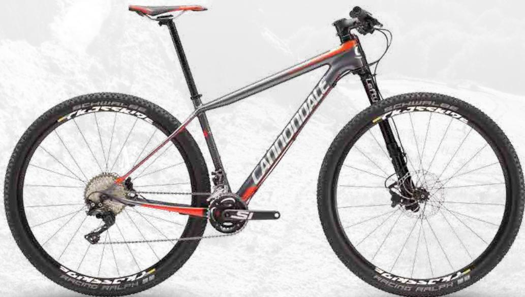
**تنه:** F-SI ASYMMETRIC, BALLISTEC CARBON, SPEED SAVE, PF30A, 1.5 SI HEADTUBE, 27.5» (M), 29» (L)
