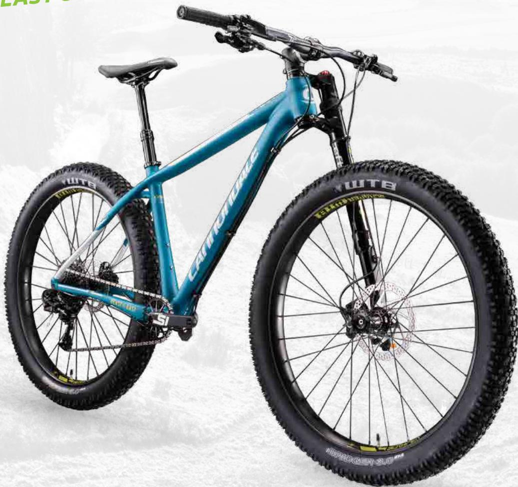
**تنه:** BEAST OF THE EAST 27+, 120mm, SMARTFORMED ALLOY, AI OFFSET, BB30, FLAT MOUNT BRAKE, 1.5 SI HEADTUBE
