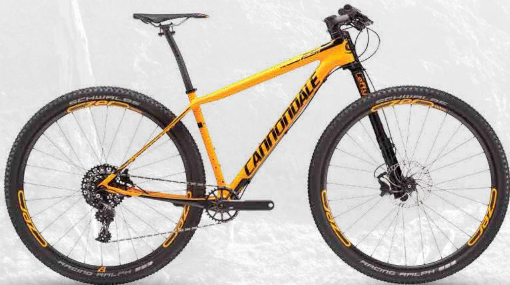
**تنه:** F-SI ASYMMETRIC, BALLISTEC CARBON, SPEED SAVE, PF30A, 1.5 SI HEAD TUBE, **27.5» (M), 29» (L)**
