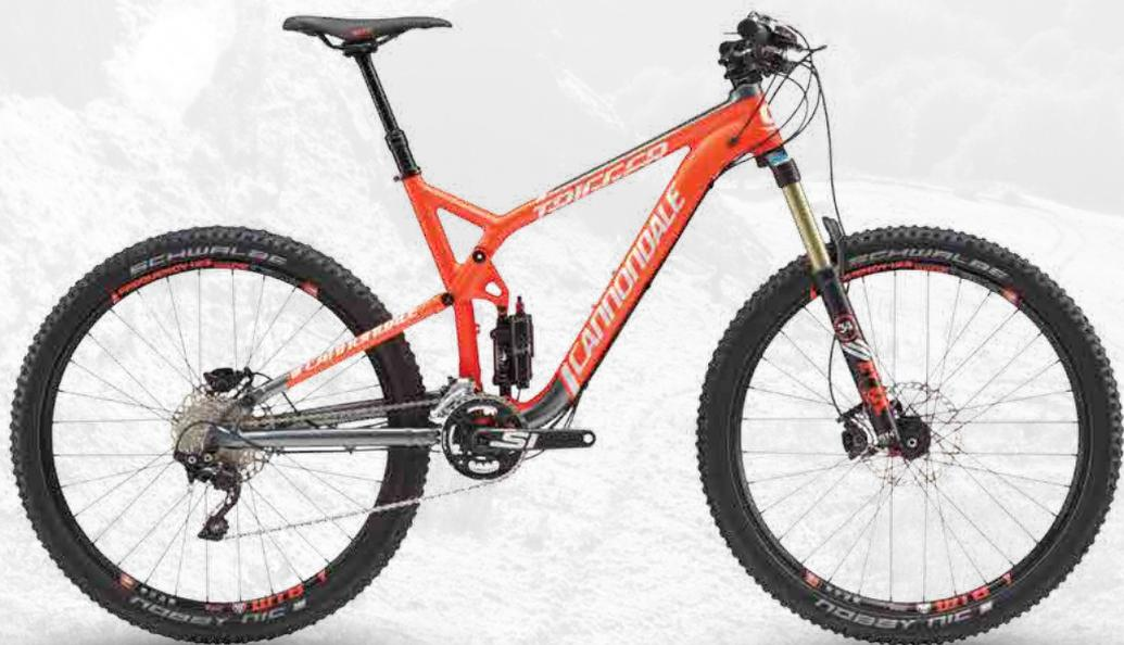
**تنه:** TRIGGER 27.5, 140/85MM, SMARTFORMED ALLOY, BB30, ISCG03, 1.5 SI HEADTUBE
